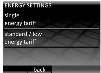
For both the standard and low energy tariff you will need to set a cost per Kilowatt hour (KWH). First set the relevant currency by pressing "up" and "down" (you can select £, \$, € and ¥). Press "ok" to proceed to the first digit of the energy tariff, press "up" and "down" to select the correct amount and then press "ok" to proceed to the second digit. Continue pressing "ok" until you have set all the digits and returned to the ENERGY MONITOR main page.
