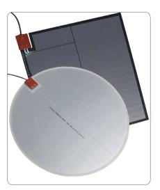
NOTE: When testing the resistance of the mirror demister allow a ±10% tolerance for pads above 25w and ±20% for pads below 25w.
